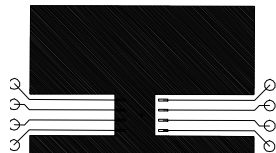
a. 50^\circ\text{C}/\text{W} on a 1\text{ in}^2 pad of 2oz copper.
